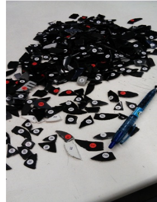
Figure 4 Labelled plastic particles for sorting test
