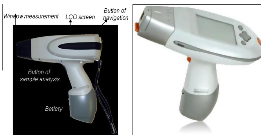
Fig. 3. Hand held XRF analyser and NIR plastic detector (Fondis electronic).
